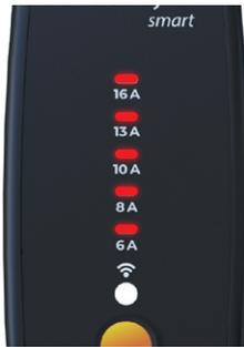
**2** Press and hold the control button for 3 seconds. This will switch the charger into the IT grid mode. The charger will restart and perform the initial self-test.
