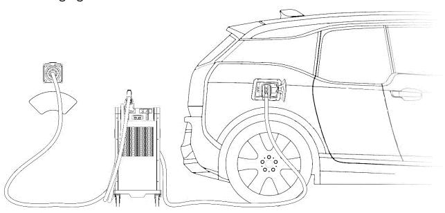
Now connect the DC plug to the vehicle. Depending on the charging procedure, fast-charging will commence automatically or you will need to press the START button on the fast-charger. During charging, you can view a range of charging information by browsing the menu structure.
