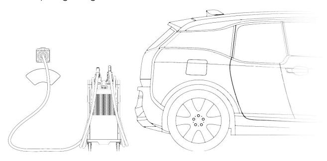
Plug the DC cable and the AC cable into the fast-charger. Now connect the AC cable to the mains supply.
