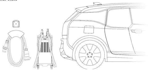
Fast charging requires a powerful mains supply, ideally a CEE 63A/400V industrial socket. Park your vehicle so the fast-charger can be connected to the mains supply using the supplied cables with the cables lying in the floor and not stretched.
